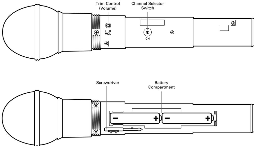
**Figure C – Handheld Transmitter**
