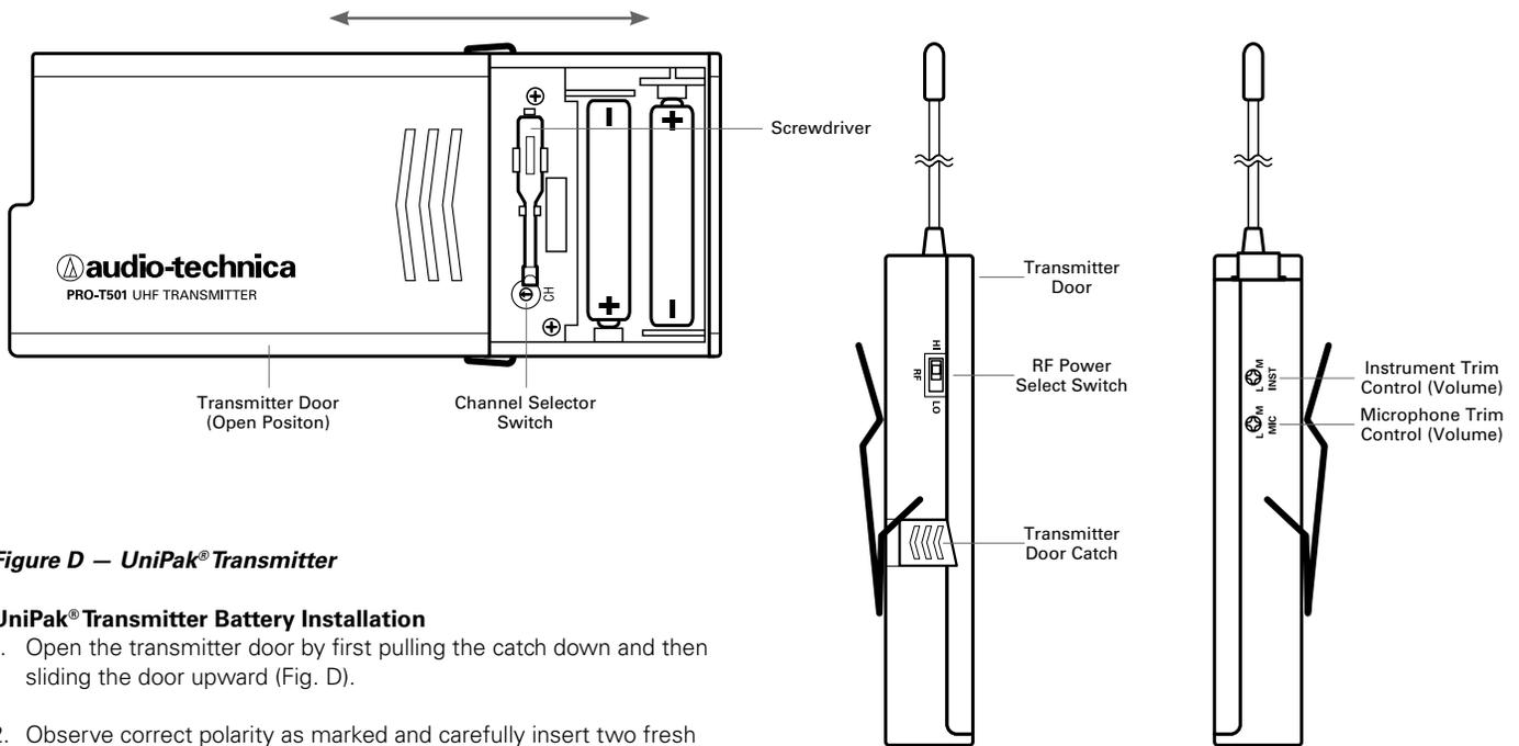
**Figure D – UniPak® Transmitter**
